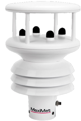
MaxiMet GMX550 measures 6 parameters including precipitation
